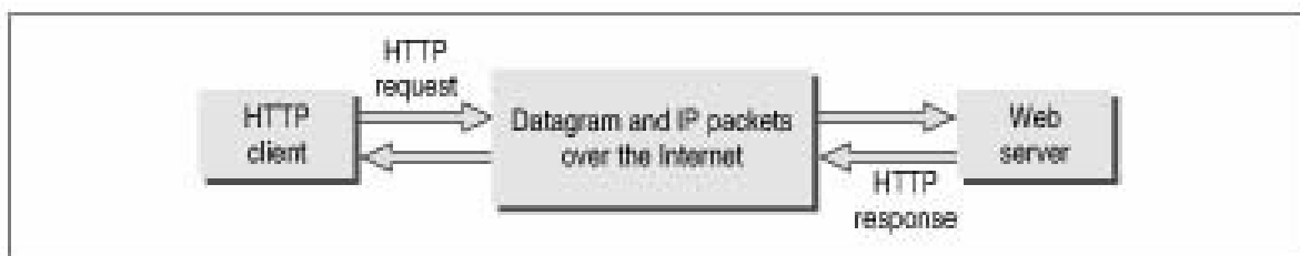
Figure 12.8 HTTP based web access architecture over the Internet
